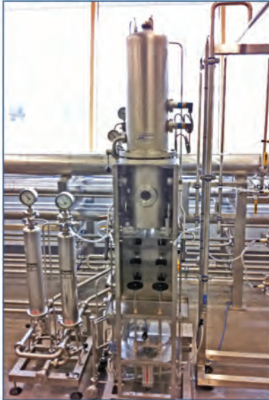
CW400 Micro Beer Carbonator, Bottling & Kegging Machine 350BPH x 500ml & 400LPH on kegging
