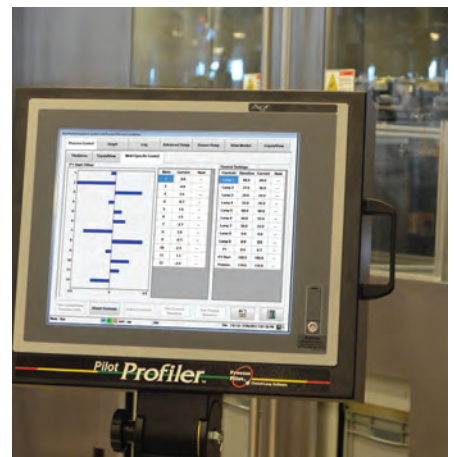
Pictured above: Individual Mold Control™ screen on Process Pilot® user interface
